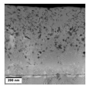
Cross-sectional transmission electron microscope image of the functionally graded smart coating with nano-silver particles distributed throughout the entire thickness of the coating. The crystalline nano-grains can be seen near the interface with the titanium implant and mostly amorphous layer on the top portion of the coating. Credit: Dr. Afsaneh Rabiei, North Carolina State University
