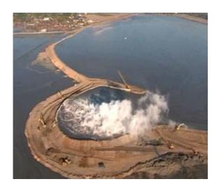
Aeriel view of the Lusi mud volcano crater and the dikes and dams constructed to contain the still-oozing mud.(Courtesy of Channel 9 Australia)
