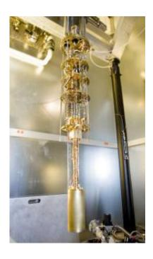
Spin qubits, which could be the core logic elements of quantum computers, are cooled in a device called a dilution refrigerator to temperatures near absolute zero in order to exploit the mysterious rules of quantum mechanics. Photo: Princeton University/Brian Wilson
