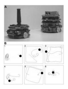
A) The predator robot (right) facing the prey robot (left). B) Six examples of pursuit and evasion strategies that evolved over the 100 generations of selection in one of the replicates (see main text for description). The position of the prey at the end of the trial is indicated by the empty disk and that of the predator by the black disk (the lines in the disks correspond to the frontal directions). Image credit: doi:10.1371/journal.pbio.1000292.g004
