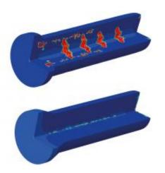
The simulation shows the results of cold forging. An optimized tool geometry (bottom) keeps pore density low. (© Fraunhofer IWM)
