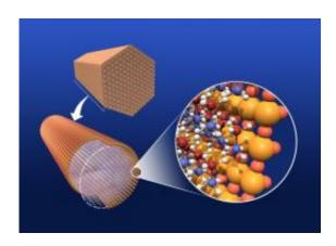
Packing ammonia borane into mesoporous silica leads to a remarkable enhancement of the hydrogen storage properties. This image shows the molecular configuration of the packed ammonia borane (while spheres are hydrogen).
