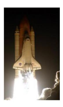
Space shuttle Endeavour lifts-off from the Kennedy Space Center at Cape Canaveral, Fla., Monday, Feb. 8, 2010. Endeavour is carrying six astronauts who will deliver a room and observation deck to the International Space Station. A piece of foam insulation is seen falling to the right of the orbiter. (AP Photo/John Raoux)
