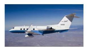
The UAVSAR pod is carried on the underbelly of NASA's Gulfstream-III research aircraft. (File Photo/NASA)
