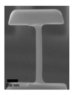
Scanning electron micrograph of a typical as-fabricated 100-nm-diameter tensile sample. Credit: Dongchan Jang/Caltech
