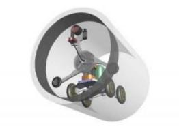
An illustration of a prototype robot that can repair damaged water pipe. Photo: Courtesy of Maria Feng / UCI
