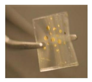
Unlike existing micromachines, the researchers' gold films are flexible, so they could be used to coat irregular surfaces. Photo: Corinne Packard
