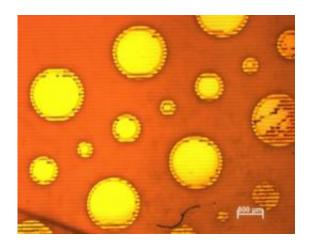
To test a new technique for creating micromachines, MIT researchers deposited films of gold on a sheet of plastic; grooves in the plastic are visible as a series of horizontal lines. Image: Corinne Packard and Apoorva Murarka
