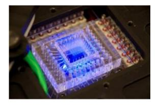
This 2 centimeter by 2 centimeter microfluidic chip is part of the SETG instrument. Tiny tubes feed in chemicals and ultraviolet light illuminates fluorescent dyes that help identify and analyze DNA. Credit: G. Ruvkun
