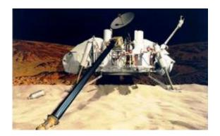
The Viking landers carried four instruments designed to search for signs of martian life: a gas chromatograph/mass spectrometer, as well as experiments for gas exchange, labeled release, and pyrolytic release. Credit: NASA
