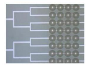
This is an example of multiple zone-plates placed over individual microfluidic channels. Credit: Laboratory of Ken Crozier, Harvard School of Engineering and Applied Sciences.
