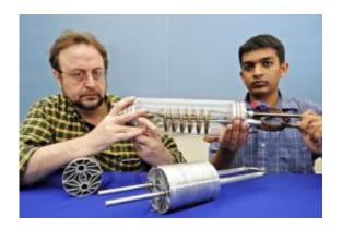
Issam Mudawar, at left, a Purdue professor of mechanical engineering, and doctoral student Milan Visaria display their first- and second-generation heat exchangers, a crucial component of a hydrogen storage system for cars. The final design is a coil of stainless steel tubing that fits inside a hydrogen storage "pressure vessel" 4 inches in diameter. Purdue has filed a final patent on the heat exchanger. (Purdue University photo/Andrew Hancock)
