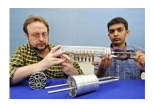
Issam Mudawar, at left, a Purdue professor of mechanical engineering, and doctoral student Milan Visaria display their first- and second-generation heat exchangers, a crucial component of a hydrogen storage system for cars. The final design is a coil of stainless steel tubing that fits inside a hydrogen storage "pressure vessel" 4 inches in diameter. Purdue has filed a final patent on the heat exchanger. (Purdue University photo/Andrew Hancock)
