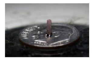
A magnetic crystal sits on the head of a dime for scale. Scientists exploit the randomness of the magnetic field in the crystal at the molecular level to control the properties of the magnet as a whole. The chip underneath the crystal is a magnetic sensor. Credit: University of Chicago
