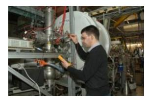
Michael Block, head of the research team, sets up the ion trap Shiptrap at GSI, where, for the first time, the mass of a super heavy element was measured. The measurement of nobelium (element 102) yielded an unprecedented accuracy. Credit: G. Otto, GSI Helmholtzzentrum für Schwerionenforschung
