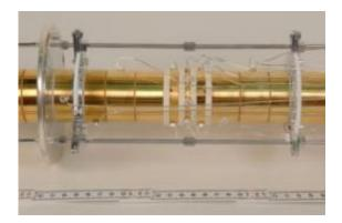
The picture shows the Penning trap, which is part of the Shiptrap experiment. A magnetic field parallel to the tube forces the arriving ions onto a spiral course inside the tube. The ions' spiraling frequency is used to directly calculate their atomic mass. The Penning trap is located inside the white tank that can be seen in picture 1. Credit: G. Otto, GSI Helmholtzzentrum für Schwerionenforschung
