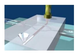
(PhysOrg.com) -- A European research project has shown how to build optical sensors directly into the structure of labs-on-chips. The breakthrough paves the way for on-the-spot medical diagnostics.
