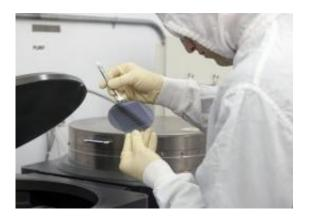
Hawkins removes a wafer containing 49 virus-detecting chips from an etching machine.
