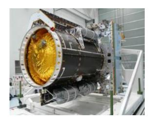
The Alphabus Service Module on the turnover trolley just before closure of the container. The spacecraft is lowered vertically on the turnover trolley, tilted horizontally, then the whole assembly is slid into the container and closed. Credits: Thales Alenia Space
