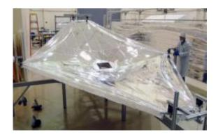
This is a photo of the 1/3 scale sunshield membranes undergoing final inspection at the Nexolve facility in Hunstville, Ala. The full-scale sunshield will fly on NASA's James Webb Space Telescope in 2014. Credit: Nexvolve
