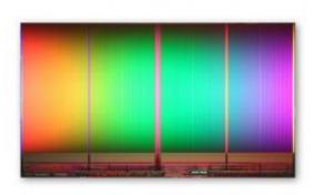
The Intel-Micron 25-nanometer (nm) 8 gigabyte (8GB) NAND flash memory device measures 167mm2 and is the smallest, most advanced process technology in the semiconductor industry.
