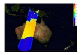
This is a calibrated image of brightness temperature over Australia. Compared to the uncalibrated image, the "noise" in the product has been reduced so that the
