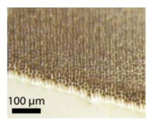
This is a photomicrograph of a silicon wire array embedded within a transparent, flexible polymer film. Credit: Caltech/Michael Kelzenberg
