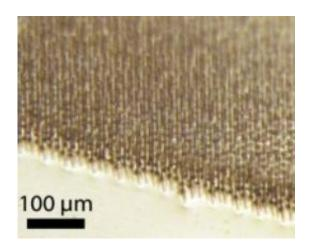
This is a photomicrograph of a silicon wire array embedded within a transparent, flexible polymer film. Credit: Caltech/Michael Kelzenberg
