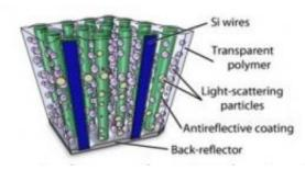
This is a schematic diagram of the light-trapping elements used to optimize absorption within a polymer-embedded silicon wire array. Credit: Caltech/Michael Kelzenberg
