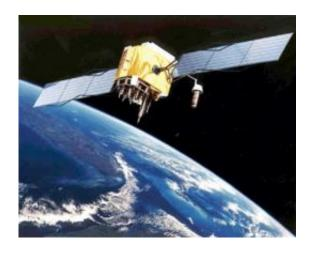
GPS is a navigation system of more than 30 satellites circling the earth. These satellites transmit signals to receivers on land, sea and air. The GPS receiver uses these signals to triangulate their exact position anywhere on the planet.
