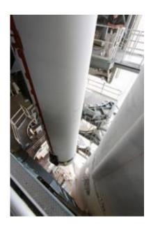
In the mobile service tower at Launch Complex 37 on Cape Canaveral Air Force Station in Fla., a solid rocket booster for the Delta IV rocket, slated to launch NASA's GOES-P satellite as it is lowered toward the base of the rocket. Credit: NASA/Jack Pfaller
