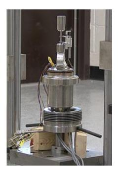
Located in a new, state-of-the-art NIST test facility, this specially designed chamber holds samples of pipeline, valve or delivery device materials for testing under pressure to determine their reaction to hydrogen. Credit: Burrus/NIST
