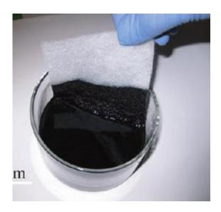
Recipe for conductive textile: Dip cloth in nanotube ink, dry in oven for 10 minutes at 120 degrees Celsius.
