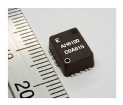
Epson Toyocom Corporation, the leader in crystal devices, today announced the development of the AH-6100LR, the world's smallest 6-axis sensor. This low-noise, low-power product comprises a 3-axis QMEMS quartz gyro-sensor and an extremely stable 3-axis accelerometer within a single package.
