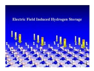
This image illustrates that an applied electric field polarizes hydrogen molecules and the substrate, inducing hydrogen absorption with good thermodynamics and kinetics. Credit: Image courtesy of Qian Wang, Ph.D./VCU.
