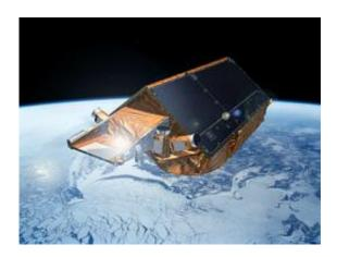
CryoSat will provide data to determine the precise rate of change in the thickness of the polar ice sheets and floating sea ice. It is capable of detecting changes as little as 1 cm per year. The information from the CryoSat will lead to a better understanding of how the volume of ice on Earth is changing and, in turn, a better appreciation of how ice and climate are linked. Credits: ESA - P. Carril
