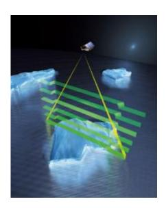
Using a sophisticated radar altimeter called SIRAL (Synthetic Aperture Radar Interferometric Radar Altimetry), CryoSat-2 will make accurate measurements of the thickness of floating sea-ice so that seasonal to inter-annual variations can be detected. It will also survey the surface of continental ice sheets to detect small elevation changes. Credits: ESA - AOES Medialab
