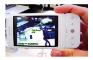
Using his mobile phone as a display and control mechanism, the resident can control the energy consumption of his appliances. (© Fraunhofer FIT)
