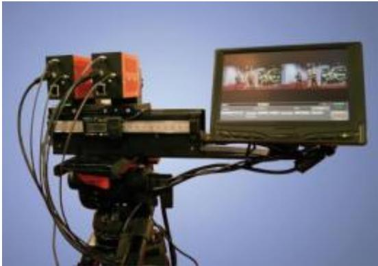
Two synchronized MicroHDTV cameras from IIS record the scene that is then transmitted in 3-D. Credit: Fraunhofer IIS
