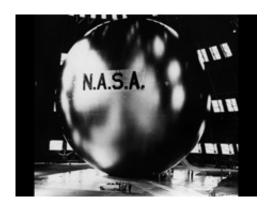
NASA's first communication satellite, Echo, was a giant mylar balloon, 100 feet in diameter, that could "bounce" a radio signal from one ground station to another. Credit: NASA
