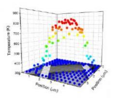
Heat transfer from biased graphene into an underlying substrate can be much higher than that found in conventional silicon transistors.
