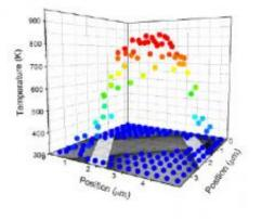
Heat transfer from biased graphene into an underlying substrate can be much higher than that found in conventional silicon transistors.
