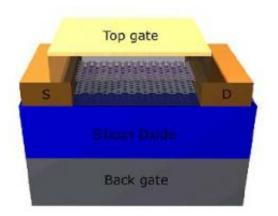
Image depicts carbon-based semiconductor chips with its dual-gate bi-layer graphene field-effect transistors.
