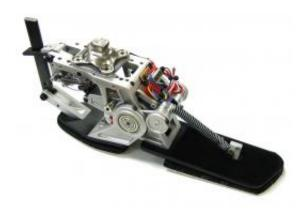
In this energy-recycling foot, the University of Michigan engineers put wasted walking energy to work enhancing the power of ankle push-off. Photo credit: Steve Collins.
