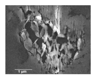
Secondary electron image of the Coki section analyzed in this study showing mineral shards surrounded by compressed aerogel.
