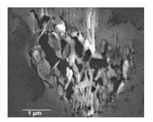
Secondary electron image of the Coki section analyzed in this study showing mineral shards surrounded by compressed aerogel.
