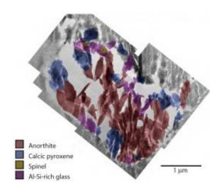
Corresponding false color mineral map overlaid on a montage of brightfield Transmission Electron Microscope (TEM) images.
