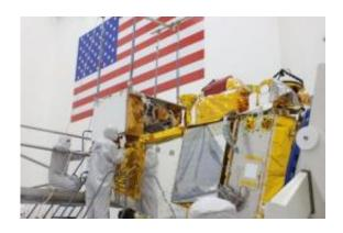
The Visible Infrared Imaging Radiometer Suite (VIIRS) arrives and begins integration with the National Polar-orbiting Operational Environmental Satellite System (NPOESS) Preparatory Project (NPP) spacecraft at Ball Aerospace in Boulder, Colo. Credit: Ball Aerospace
