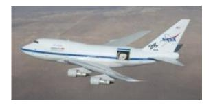
SOFIA in flight with telescope's door wide open.
