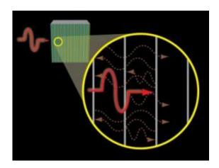
At the boundaries between layers, the photon creates waves interfering with each other, affecting its transit time. Credit: JQI
