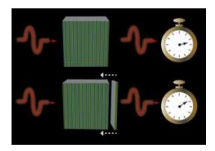
A single photon travels through alternating layers of low (blue) and high (green) refractive index material more slowly (top) or quickly (bottom) depending upon the order of the layers. A strategically placed additional layer (bottom) can dramatically reduce photon transit time. Credit: JQI
