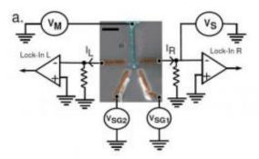
This is an SEM image of a typical Cooper pair splitter. The bar is 1 micrometer. A central superconducting electrode (blue) is connected to two quantum dots engineered in the same single wall carbon nanotube (in purple). Entangled electrons inside the superconductor can be coaxed to move in opposite directions in the nanotube, ending up at separate quantum dots, while remaining entangled. Credit: L.G. Herrmann, F. Portier, P. Roche, A. Levy Yeyati, T. Kontos, and C. Strunk
