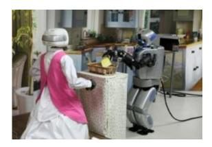
Mahru-Z (R), a robot developed by the Korea Institute of Science and Technology picks up a sandwich in Seoul. South Korean scientists have developed a walking robot maid which can clean a home, dump clothes in a washing machine and even heat food in a microwave. The institute took two years to develop Mahru-Z.
