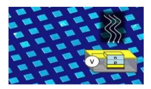
The self assembly process made a device of 64,000 parts in 3 minutes. Image: Heiko O. Jacobs
