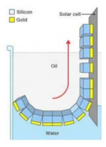
The self assembly process. Elements align at the oil/water boundary. The "blank" solar cell has pre-cut places for the elements and is dipped through the boundary. As it is slowly drawn upwards, the elements pop into place. Image: Heiko O. Jacobs.
