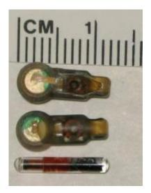
Two tags from the Juvenile Salmon Acoustic Telemetry System sit above a tag from the widely used Passive Integrated Transponder fish tracking system. Credit: Pacific Northwest National Laboratory
