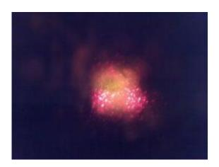
This microscope image shows a portion of a piece of an electrically conducting plastic or polymer film that has been bombarded by a pulse of green light from a conventional laser. The green light excites tiny cavities within the film to produce red-colored "random laser" light seen in the photo. University of Utah physicists have published a study explaining how this bizarre kind of laser works. Credit: Randy Polson, University of Utah.
