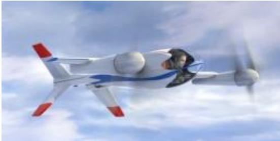
(PhysOrg.com) -- NASA engineers have designed an extremely quiet one-person electrically powered aircraft that can hover like a helicopter and fly like a plane. The “Puffin” launches from an upright position with the tail split into four legs that serve as stable landing/take-off gear.
