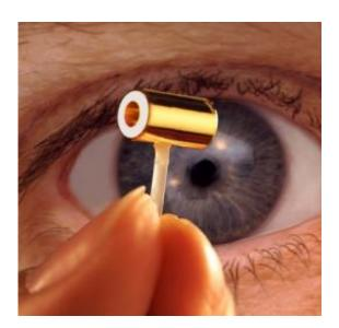
A tiny chamber made of gold, called a hohlraum, is used to contain the pellet of heavy hydrogen fuel at the center of a fusion reaction at the National Ignition Facility. Laser beams enter through the two open ends of the hohlraum and are reflected in toward the fuel, heating it up to produce the fusion reaction. Image: National Ignition Facility
