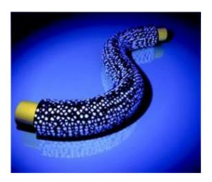
Scientists have developed coaxial nanocables: carbon nanotubes coated with titanium dioxide. Image credit: Cao, et al. (c)Chemistry of Materials.
