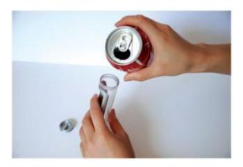
As Zheng explains, a sugar-powered phone could potentially offer a much more environmentally friendly power source than lithium ion batteries. The new phone's bio battery, which basically acts as a <u>fuel cell</u>, uses enzymes as the <u>catalyst</u> to generate <u>electricity</u> from carbohydrates.
