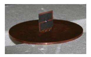
This Z antenna tested at the National Institute of Standards and Technology is smaller than a standard antenna with comparable properties. Its high efficiency is derived from the "Z element" inside the square that acts as a metamaterial, greatly boosting the signal sent over the air. The square is 30 millimeters on a side. Credit: C. Holloway/NIST
